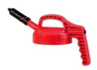
The OilSafe Mini Spout Lid has an outlet diameter of 1/4" (7mm), making it ideal for lubrication jobs where equipment fill holes are small such as constant level oilers and machine tools.
